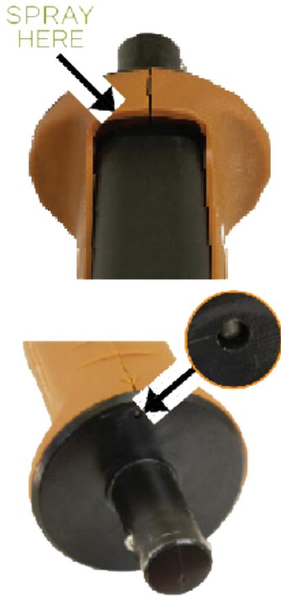
1. Pull the trigger in and spray a silicone based lubricant into the hollow area. Pull the trigger again several times in order to spread the lubricant.
