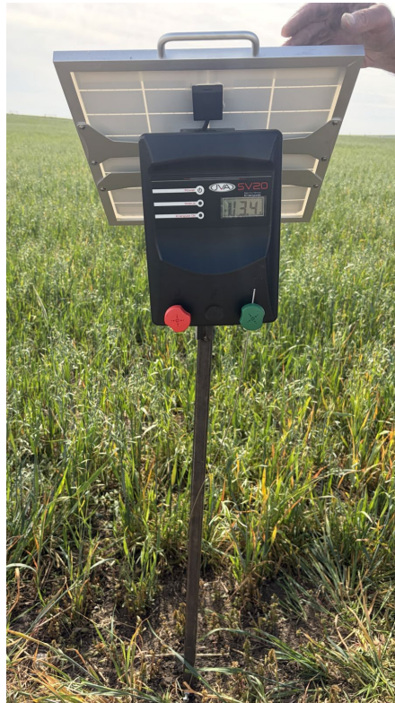
Energizer mounted, grounded and facing south.
